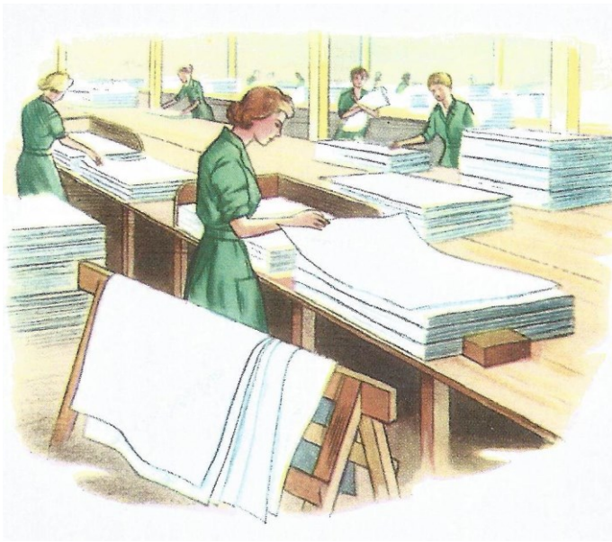
Sheets of paper produced at Aylesford are inspected in the new salle. The girls also count the sheets in reams
